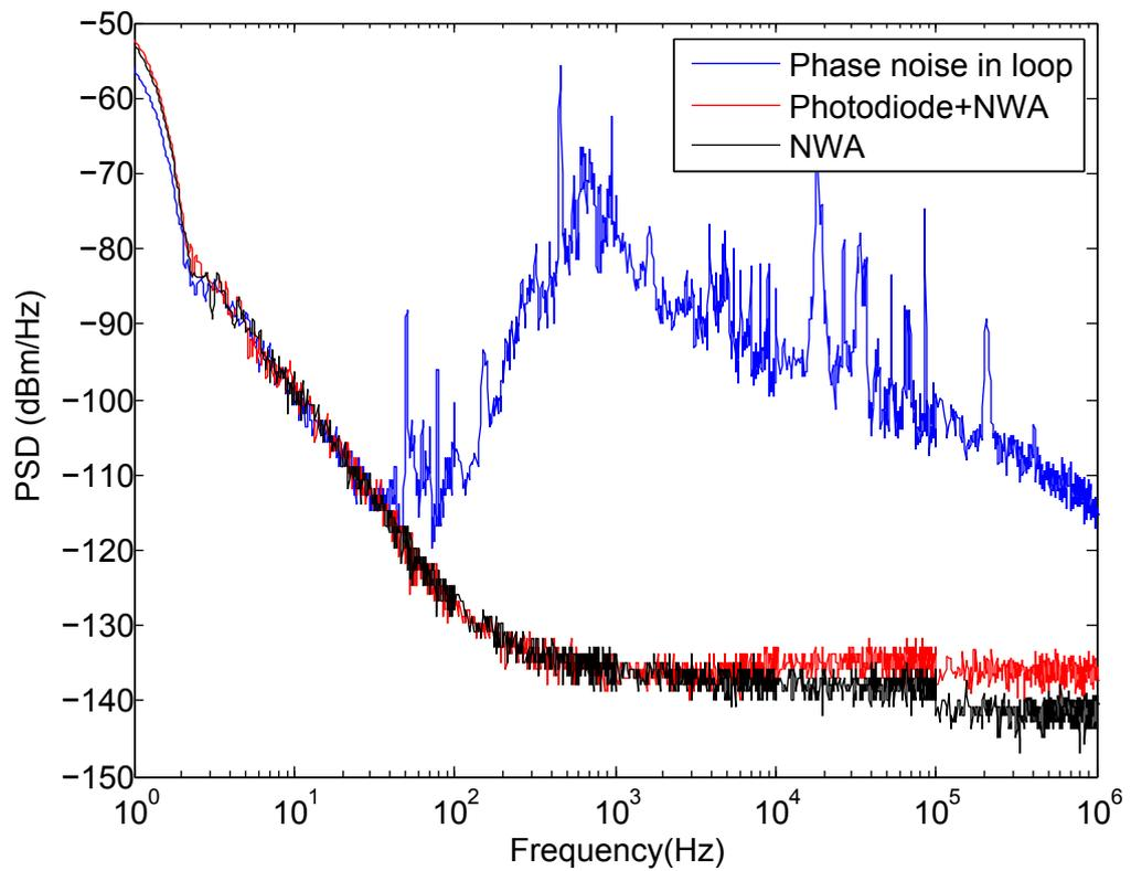
**Fig. 3.7:** PSD of the common mode phase noise in loop due to the common mode movement of the optical lattice. Moreover the corresponding noise floor the network analyzer and of the photodiode, which also contains the NWA noise floor was measured.
