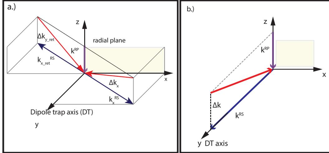
**Fig. 2.16:** Illustration of the momentum kick for both configurations. a.) shows the first attempt. b.) Used Configuration for cooling into the ground state
