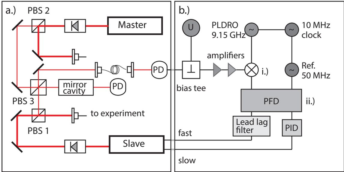
**Fig. 2.9:** Raman Setup for the stabilization of the phase (frequency) difference between both lasers. The phase of the ‘slave’ laser is stabilized to the one of the ‘master’ laser in the optical phase lock loop (OPLL).
