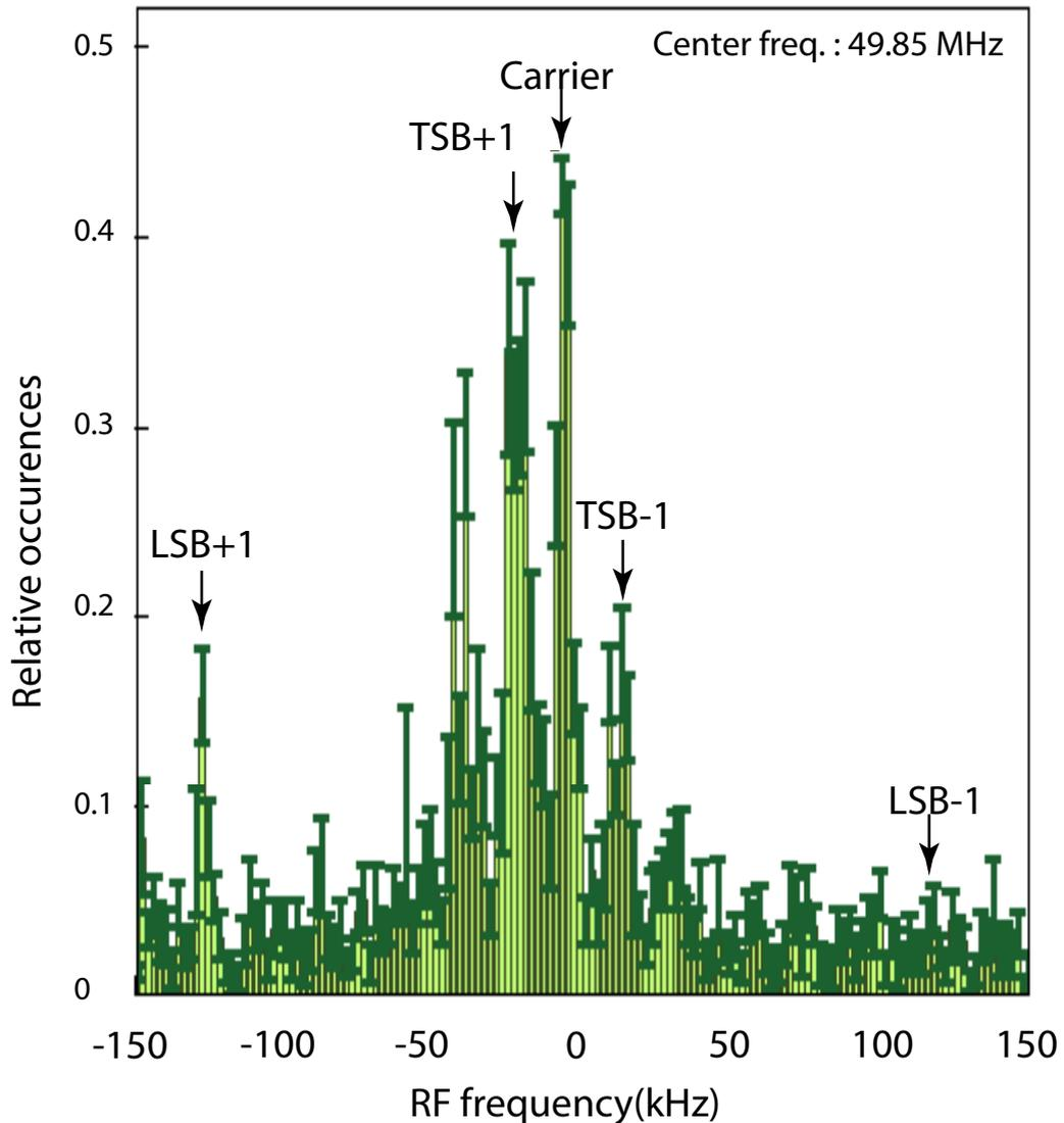
**Fig. 2.20:** Demonstration of cooling into the motional ground state. The whole spectrum is shown. The transversal sidebands are as expected separated from the carrier frequency at  $\pm 49.85$  MHz by  $\approx \pm 20$  kHz. At 110 kHz from the carrier the first longitudinal heating sidebands appear. [With kind permission by C. Robens]
