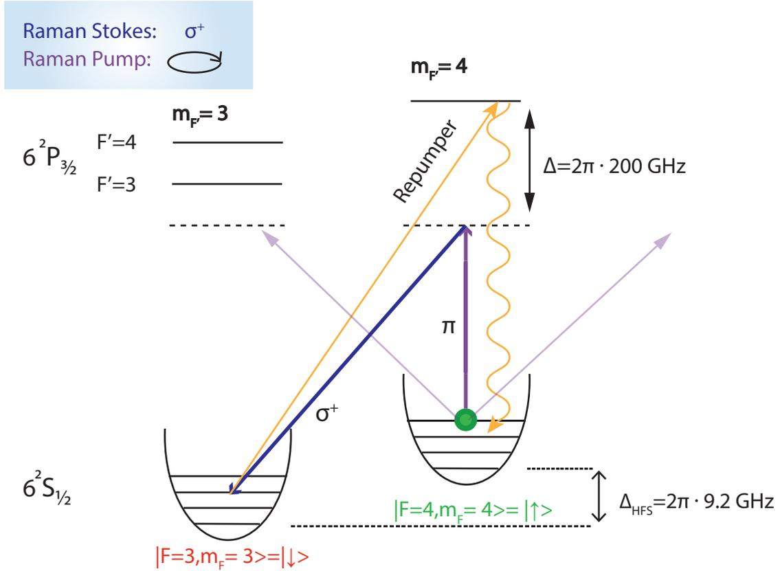
**Fig. 2.19:** Illustration of the configuration of used transitions for our Raman sideband cooling scheme.
