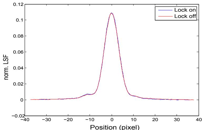
**Fig. 3.13:** This graph displays the normalized LSF both when the feedback was turned on and off. For the case out of loop the FWHM was at 7.713 px [2.234 microns] with a strehl ratio of 0.771. In case with the feedback loop we obtained for the FWHM 7.778px[2.252 microns] and a strehl ratio of 0.772. The FWHM for the case in loop is slightly higher since the sensitivity to the phase noise is higher. %
