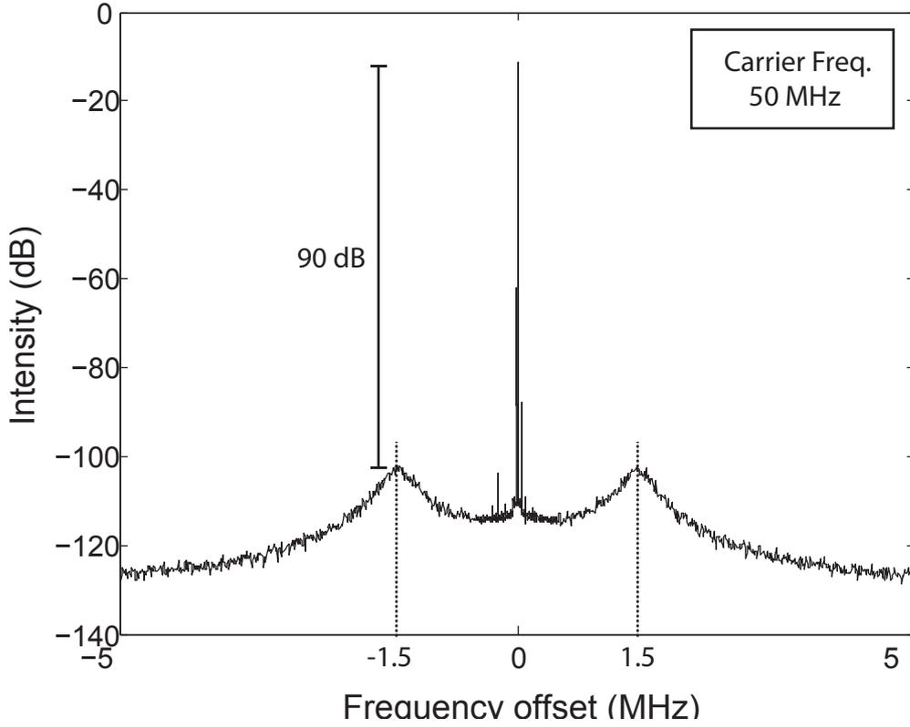
**Fig. 2.10:** Spectrum of the signal of the OPLL. The x-axis shows the offset from the central (carrier) frequency of 50MHz. The amplitude ration between the carrier and the servo bumps is at 90 dB. The characteristic peaks, called servo bumps, are at 1.5 MHz. They determine the working range of the feedback loop and arise from phase differences that they are not compensated but enhanced by the PFD [47].
