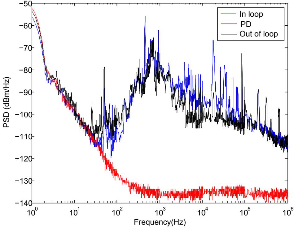
**Fig. 3.9:** Noise from the light field of the dipole trap in the unlocked and the locked case. Since the lock increases the sensitivity for the noise the amplitude from the measurement with a lock is increased by 3 dBm/Hz (c.f. Tab 3.1).
