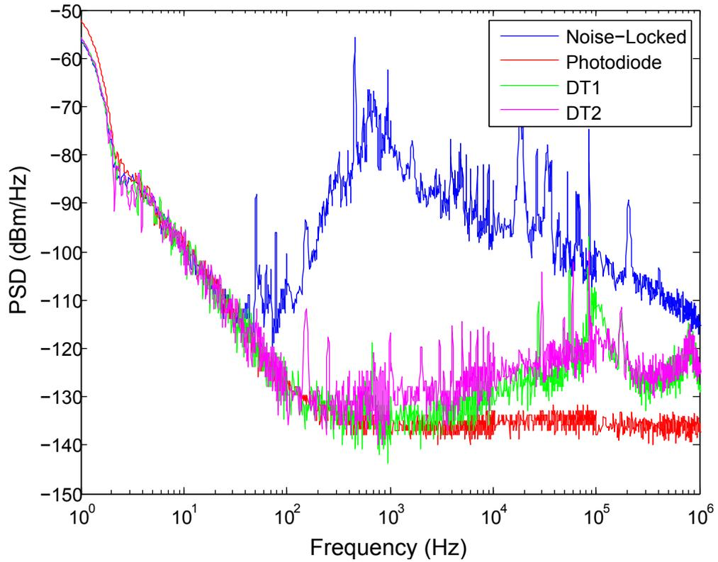
**Fig. 3.8:** The noise signal is plotted together with the PSD spectrum from DT1 and DT2. The amplitude of the measurement with the interferometer is well above the contribution from DT1 and DT2. For low frequencies (<1 kHz) the amplitude from DT1 and DT2 is on the background noise level. Both arms own a very similar noise behaviour over the whole frequency range
