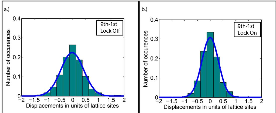
**Fig. 3.15:** Histogram and gaussian fit for the displacement from atoms from the first and the last (ninth) image in one sequence without (a.) and with(b.) the loop turned on. The time between these images was 36s which is the largest time distance. One can see that the lock minimized the spatial drift of the optical lattice ( $\approx 30\%$ ) A similar distribution to the first case is recovered by the loop.
