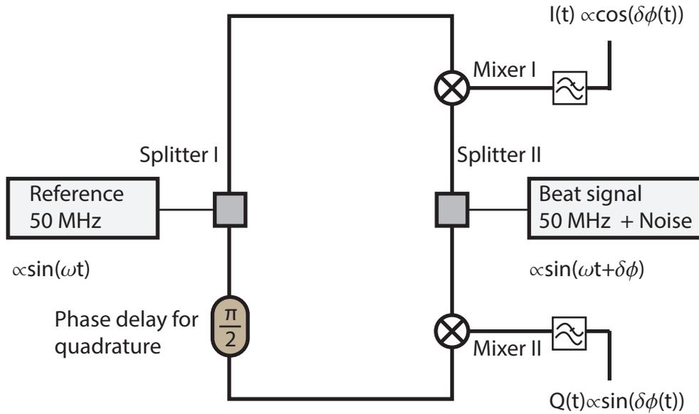
**Fig. 2.11:** Schematic draft of the experimental setup for the quadrature measurement. The beat signal is split into two arms. For the creation of the quadrature component an additional phase delay of ideally  $\frac{\pi}{2}$  is added. Each arm is then mixed with a reference signal, forming the In-phase component  $I(t) \propto \cos(\delta\phi(t))$  and the quadrature component  $Q(t) \propto \sin(\delta\phi(t))$ . Lowpass filters suppress the sum term.
