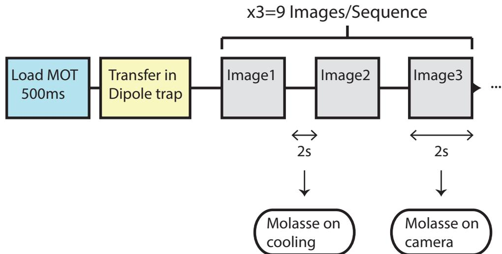
**Fig. 3.11:** Schematic representation of one experimental sequence for obtaining the images. Each sequence produced 9 images, was repeated 1000 times. Thus it resulted in a total of 9000 images. This was done with and without lock. In order to have only few Atoms, atoms are loaded into the MOT for 500ms, then transferred into the dipole trap, and then the first image is taken. Referring to this taking an image and the break in between tooks 2s each.
