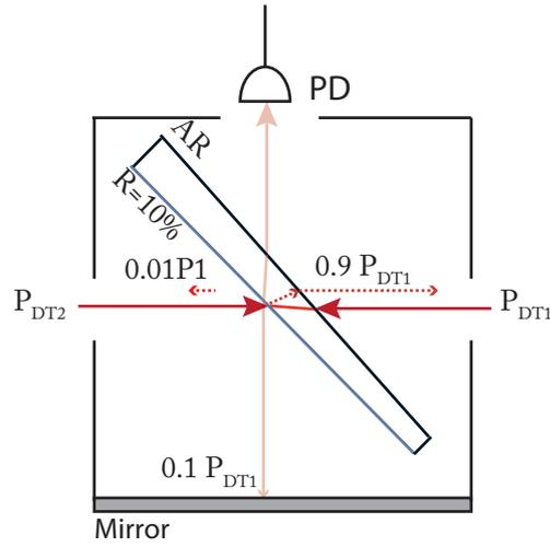
**Fig. 3.3:** Schematic of the interferometer cube showing the beam path and the corresponding fractions of the beam powers creating the beat signal
