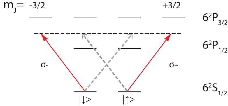
**Fig. 2.3:** The 'mixed' polarization components of the potential cancel by being equally blue(red) detuned to the 'magic' wavelength of 865.9 nm. The remaining dipole transitions are red detuned and lead to an attractive potential [adapted from [23]]
