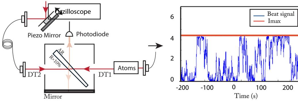
**Fig. 3.5:** a.) Schematic of the setup to measure temporal drifts. The piezo mirror controls the optical phase of DT2. The interference signal is recorded by a photodiode and displayed by an oscilloscope b.) Observation of temporal drifts in a time interval (8min) much shorter than the data acquisition time for later measurements (45min)
