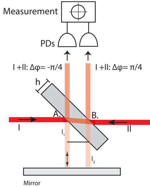
**Fig. 4.2:** Generation of the quadrature components  $I(t)$  and  $Q(t)$ . A glass plate serves as a beam splitter. The phase delay  $\Delta x$  corresponds to a delay of  $\frac{\pi}{4}$ . Both beams accumulate this delay. Since they are counterpropagating the relative phase delay results in  $\frac{\pi}{2}$ .
