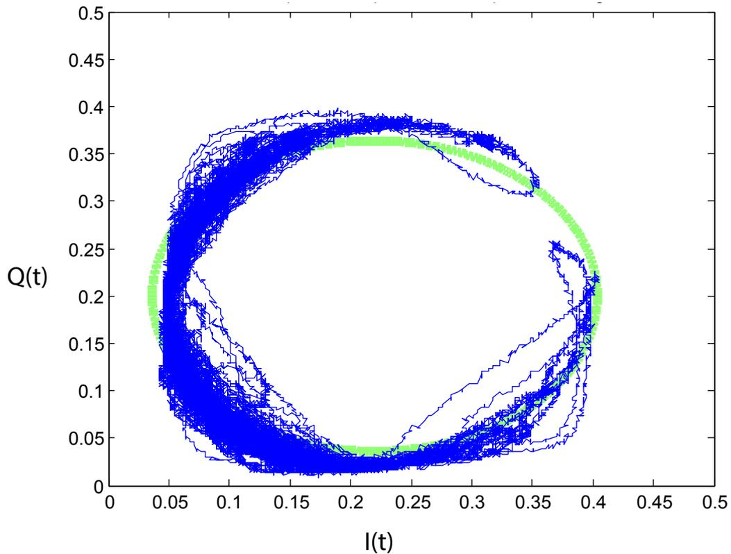
**Fig. 4.3:** Measurement of the temporal drifts of the quadrature signal. The signal is drifting along an elliptical trajectory. Fluctuations in the amplitude of  $I(t)$  ( $Q(t)$ ) lead to the broadening of the line in both directions. The signals are not in quadrature which leads to the elliptical shape and the offset from the zero line.
