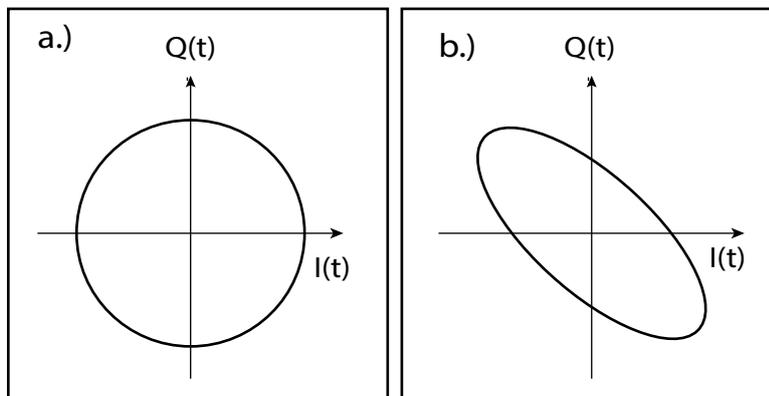
**Fig. 2.12:** Demonstration of the change of the shape for a deviation of the relative phase difference of  $\frac{\pi}{2}$  (a.). b.) In this case there is a deviation of  $\frac{\pi}{4}$  from the perfect phase delay, yielding an ellipse.
