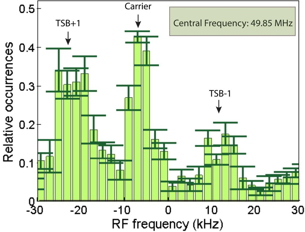
Fig. 2.21: Illustration of the carrier and the first transversal sidebands for a smaller span. [With kind permission by C. Robens]
