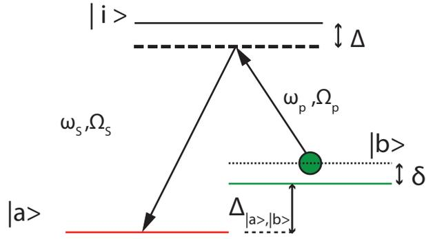
**Fig. 2.5:** The application of coherent Raman transitions couples two states  $|a\rangle$  and  $|b\rangle$  by means of an virtual state  $|i\rangle$  in a two photon process. The virtual state is far detuned from resonance in order to avoid excitation.
