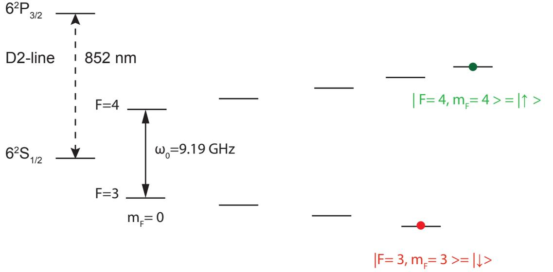
**Fig. 2.2:** Illustration of the HFS structure of  $^{133}\text{Cs}$  of the  $6^2S_{1/2}$  state with the choice of the two basis states for our experiment which are the outermost Zeeman sublevels  $|F=4, m_F=4\rangle \equiv |\uparrow\rangle$  and  $|F=3, m_F=3\rangle \equiv |\downarrow\rangle$ .
