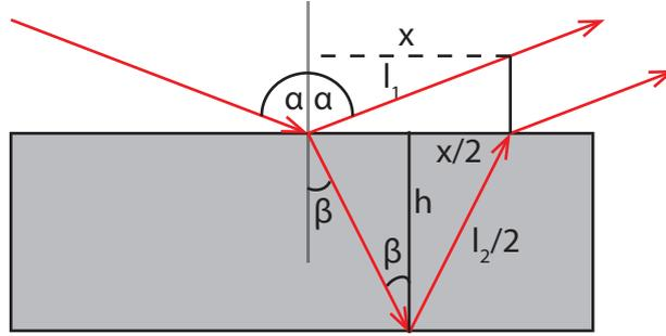
**Fig. 6.2:** Illustration for the relations used below. There  $\alpha$  denotes the incidence angle,  $h$  the thickness of the glassplate,  $\beta$  the angle in the glassplate,  $l_1$  and  $l_2$  the different path lengths.
