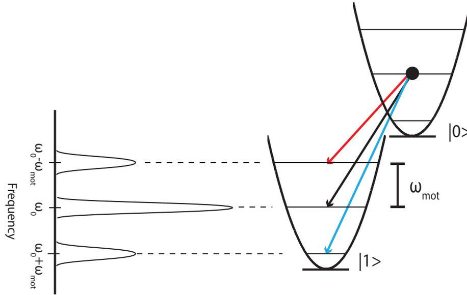
**Fig. 2.4:** Illustration of sideband transitions coupling different motional states of a two level atom in a harmonic potential. In the absorption spectrum this results in the appearance of sidebands at a distance  $\pm\omega_{\text{mot}}$  from the carrier transition with frequency  $\omega_0$  [adapted from [39]]
