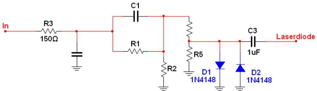
**Fig. 6.1:** Schematics of the Lead Lag Filter which increases the bandwidth of the OPLL, i.e compensates signals which are up to 1.5MHz away. This is indicated by the servobumps at this frequency(c.f Fig.???. Schematics are after [47, 48]
