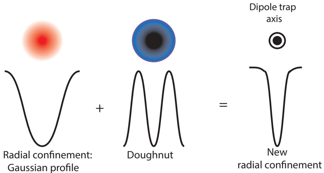
**Fig. 2.8:** Implementation of a doughnut shaped blue detuned laser beam increases the radial confinement. b.) The confinement has been increased compared to Fig.2.7
