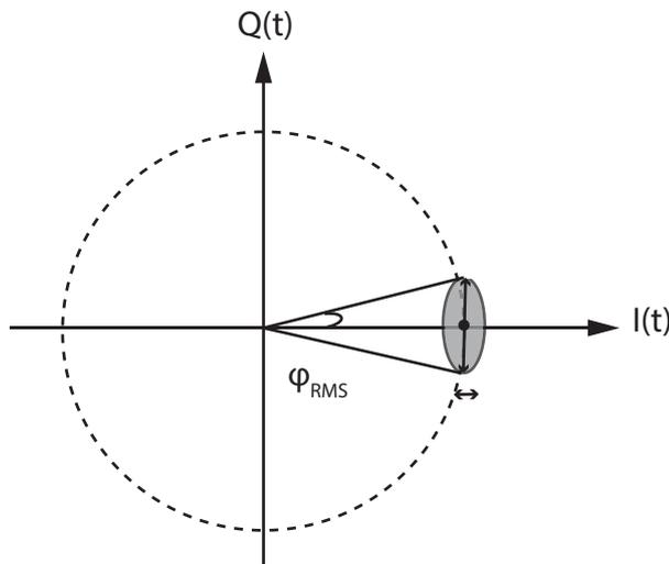
**Fig. 2.13:** a.) shows a sketch of a quadrature signal with noise in the I(t) and Q(t) branch as it was adjusted for measurement
