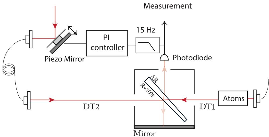
**Fig. 3.6:** Setup of the addition of the system for compensation of the temporal drifts shown in Fig.3.5. It consists of a low pass filter to generate a slow loop and the corresponding PI control. The signal from the photodiode serves as an error signal. The output of the PI control is the input of the piezo mirror.
