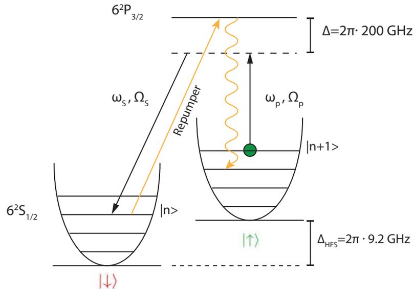
**Fig. 2.6:** Raman sideband transitions between the basis states of our experiment denoted by  $|\uparrow\rangle$  and  $|\downarrow\rangle$ . The Raman pump laser is tuned to the first blue sideband which lowers the motional state by one when the atom is transferred into  $|\downarrow\rangle$ . For cooling a repumper and spontaneous emission transfer the atom into the initial state.
