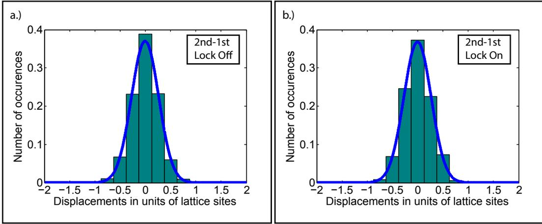
**Fig. 3.14:** Histogram and a gaussian fit for the displacement of an atoms position from the first to the second image without a.) and with the feedback loop. The time difference between the compared images was 4 s. The distributions are clearly peaked at zero (Tab.3.2).
