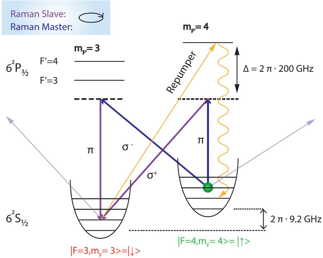
**Fig. 2.17:** Illustration of the Raman sideband cooling in the first attempt. The RP beam is tuned to the first blue sideband. The Raman pump (RP) and the Raman Stokes (RS) laser are detuned by  $\Delta$  from the D2 line of cesium. The atom, initially in  $|\uparrow, n+1\rangle$  is pumped to the intermediate state. Then stimulated emission by the RS beam transfers the atom into  $|\downarrow, n\rangle$ . A repumper transfers the atoms to the  $|\uparrow, n\rangle$  state.
