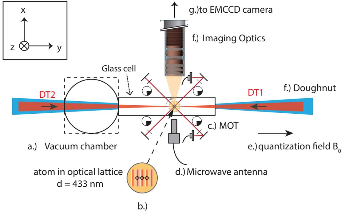
**Fig. 2.14:** Experimental apparatus for cooling and trapping the cesium atoms. For simplicity only the main components are shown. a.) Vacuum chamber with attached glass cell b.) State dependent optical lattice by dipole trap arm one (DT1) and DT2 respectively c.) Magneto optical trap (MOT) d.) Microwave antenna e.) Quantization axis by guiding field f.) Imaging optics including objective with  $NA=0.29$  [29]. g.) EMCCD camera for fluorescence detection. Further references in text.
