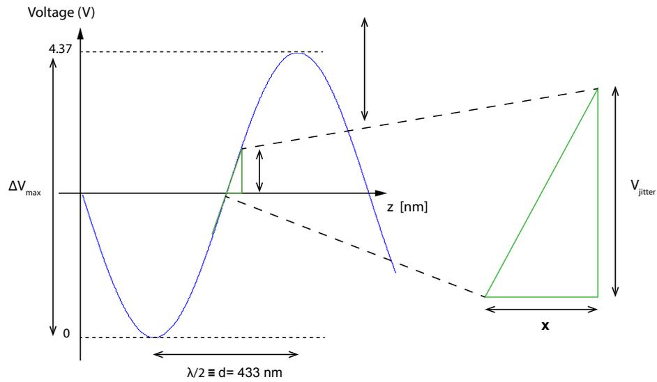
**Fig. 3.10:** Illustration for the derivation of the RMS value of the common mode phase noise in units of lattice sites  $a$ .
