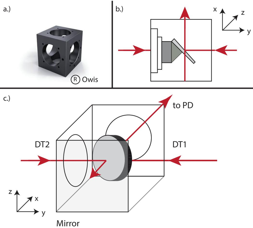
**Fig. 3.2:** Illustration of the interferometer built as a compact cube which can be mounted stable such that no additional noise is added. a.) shows an image of the cube, b.) and c.) illustrate how the wedged glass plate used for overlapping DT1 and DT2 is inserted in this cube.
