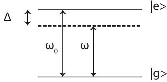
**Fig. 2.1:** Illustration of the atom as a two level quantum system with the groundstate  $|g\rangle$  and excited state  $|e\rangle$ . The frequency of the resonant transition is denoted by  $\omega_0$ , the frequency of the light field by  $\omega$  and the detuning defined as  $\Delta \equiv \omega - \omega_0$
