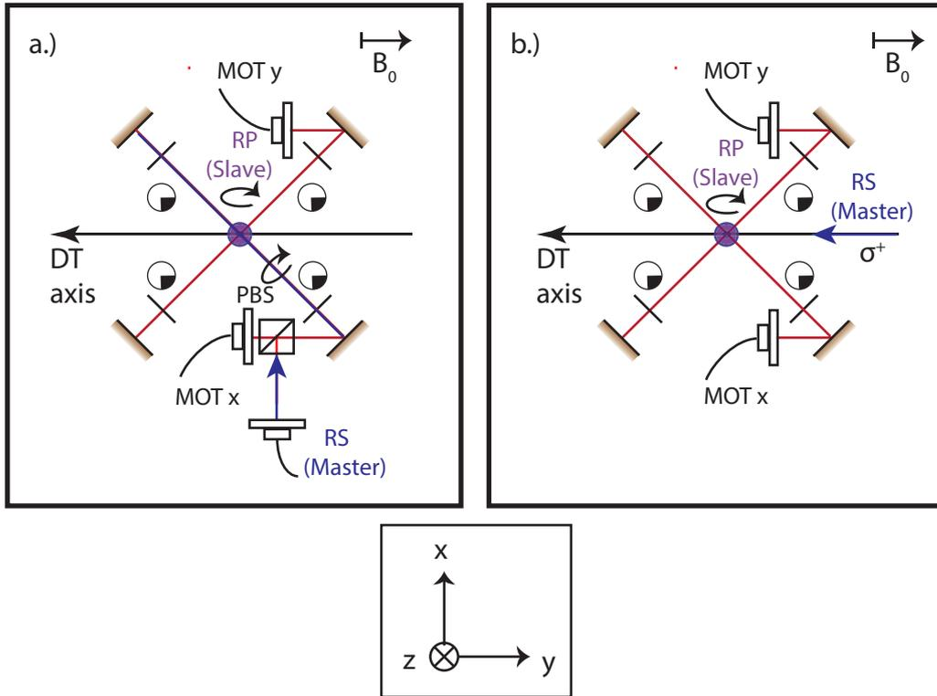
Fig. 2.15: Comparison of the two configurations. For the final cooling the b.) was used.
